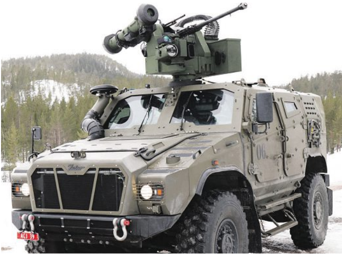
ATV 4x4 ZETOR GERLACH s RCWS KONGSBERG RS6 30x113 mm
